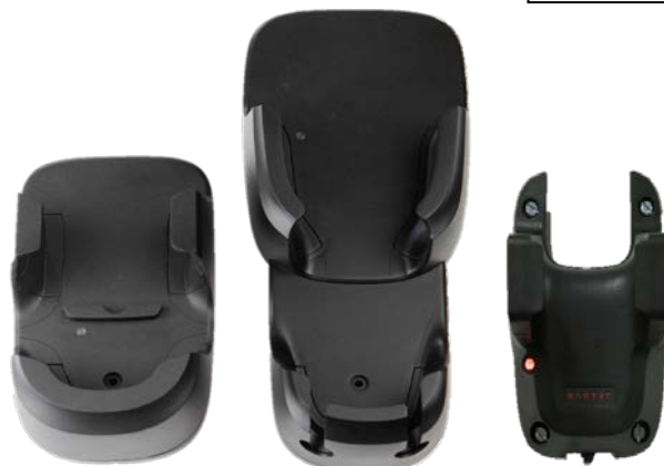
CUB Adapter programming Fixture
